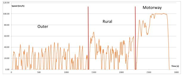
To warm the vehicle up prior to testing, only the Outer phase shall be used.
