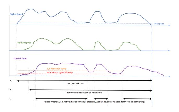
(A) Telematics data with timing period 'A' must include the sum (or average) of all key-on to key-off data over the 24 hour period (as shown by 'A' in the above timing chart).
